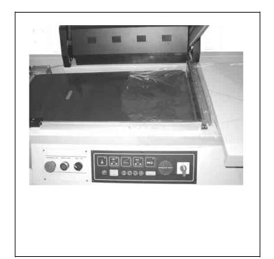
Rotate the selector (Q) to MANUALposition and press the start button (P). The machine will automatically start operating, and the first welding will be performed on the film's left side. With the right hand detach the film from the sealing blade.
