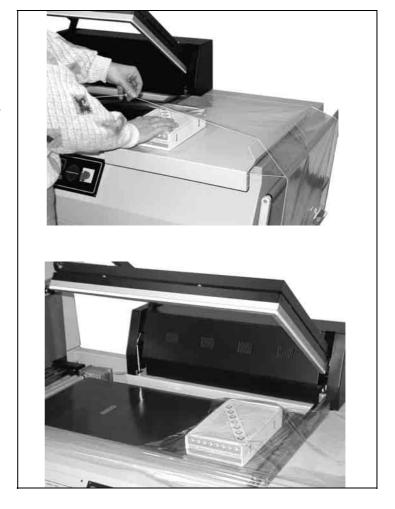
Press the ON push-button (P). The welding frame will automatically lower to cut and weld the film. When the frame opens again, the packed product will be fed towards the tunnel. Thus, the welding area will be released and ready to start a new welding cycle. If the machine is set to operate in automatic mode, it will restart work according to the rhythm set by programming.
