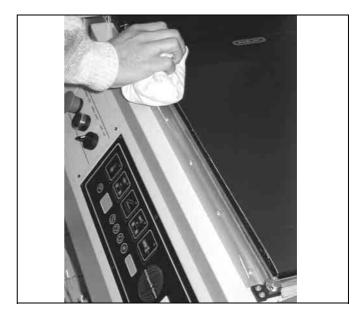
Lubricate the welding blade periodically with the supplied non-adhesive spray
