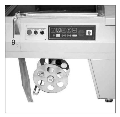
Guide this film strip around the transmission roll (9) and the driving roll (10) and couple it with the coiler (11).
